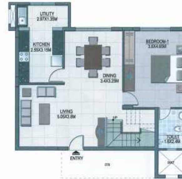
Type F1 - 3 Bedroom Duplex Ground Floor Unit Plan Unit Area - 2089 sq.ft. Core 2,3,5,6
