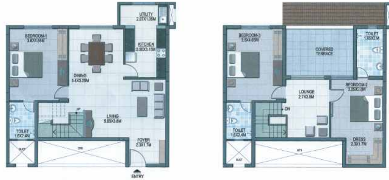
Type F - 3 Bedroom Duplex Ground Floor Unit Plan Unit Area - 2140 sq.ft. Core 1,4
